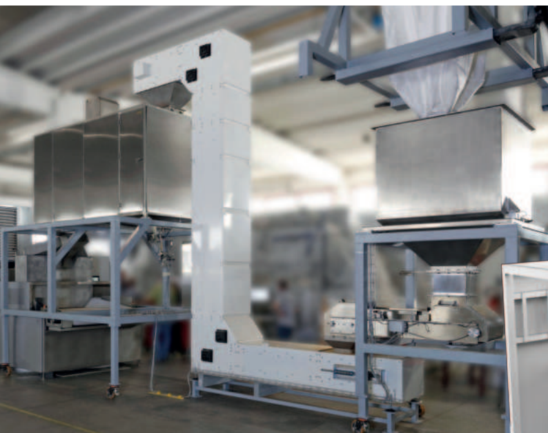
Complete line with top hopper for receiving the product, weighing belt, elevator, drum coating machine and dosing system.
