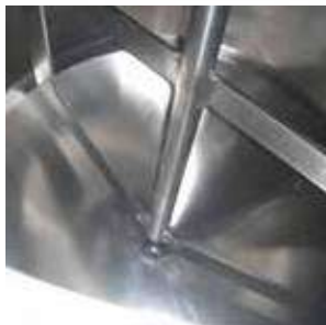
INTERNAL DETAIL OF THE MIXER WITH PTFE SCRAPING BLADES AND MIRROR-POLISHED SURFACE FINISH
