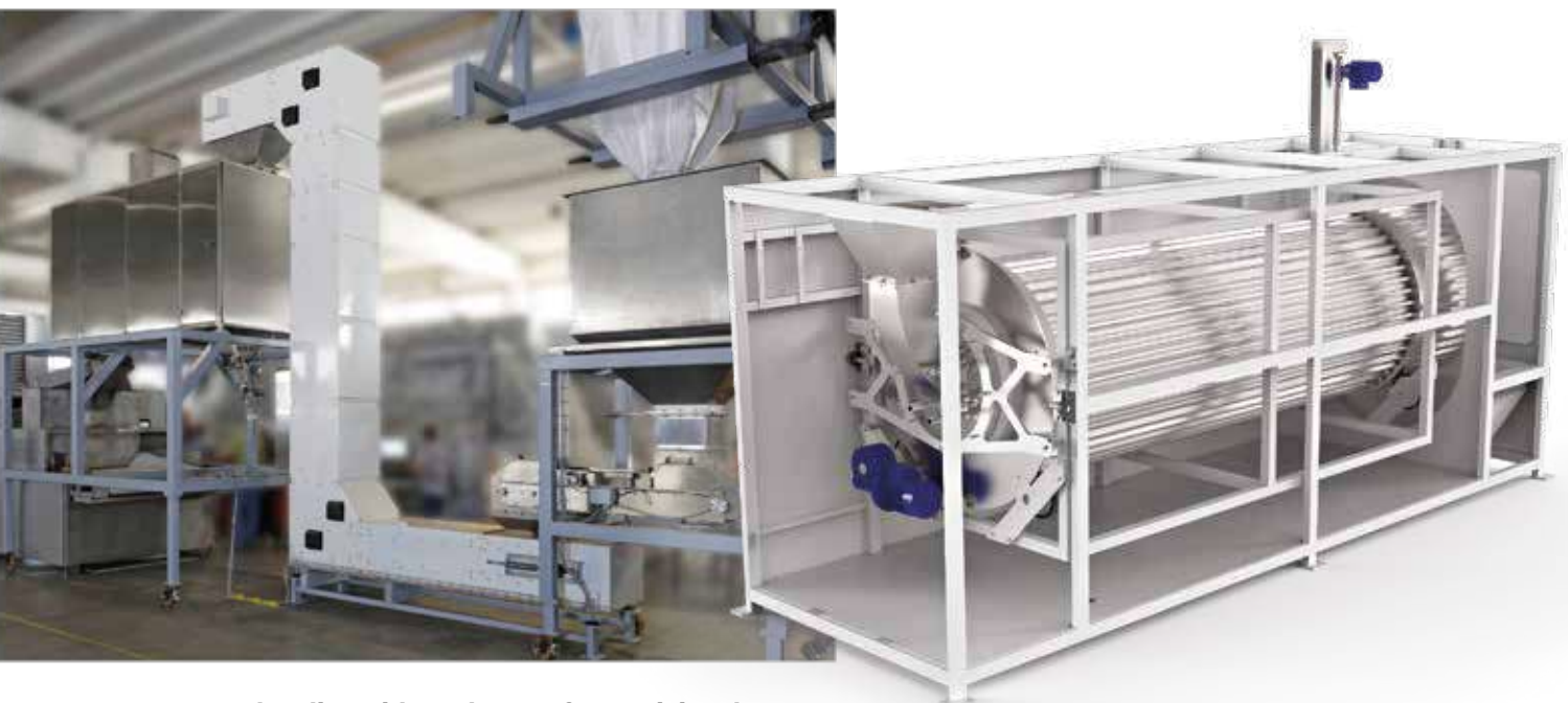
Complete line with top hopper for receiving the product, weighing belt, elevator, drum coating machine and dosing system.
