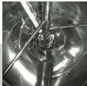
INTERNAL DETAIL OF THE ANCHOR MIXER WITH SATIN-FINISHED SURFACE
