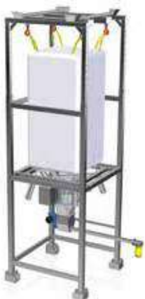
UNLOADING BIG BAG STATION, WITH DOSING SCREW
